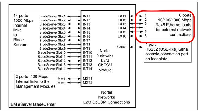
Figure 4-5 Connections on the Nortel GbESM
